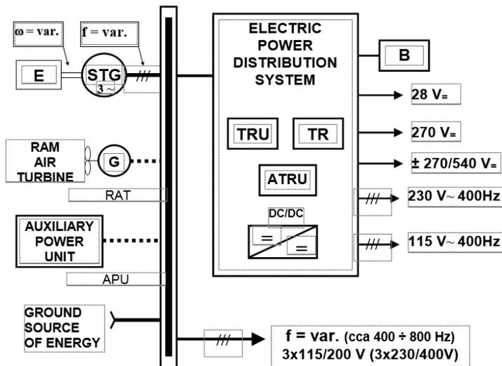
Fig. 5 The scheme of the modern aircraft electric power system
