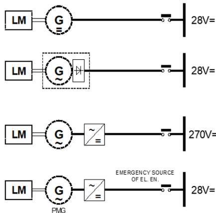
Fig. 3 Structural diagrams of DC power systems
