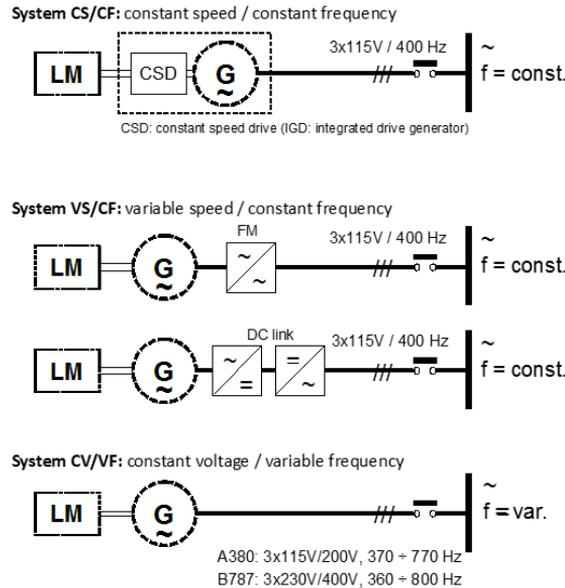
Fig. 4 Structural diagrams of AC power systems
