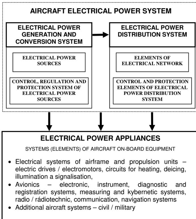
*Fig. 1 Block diagram of on-board electrical power supplying system*
