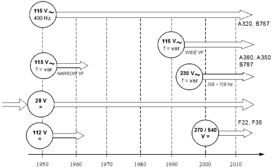
Fig. 2 Development of standardized voltage values of airborne aircraft electrical systems
