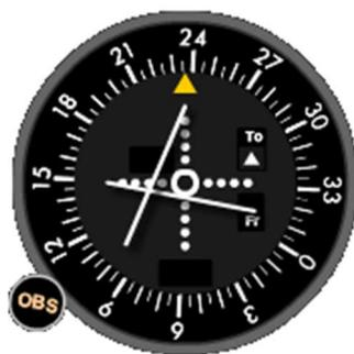
Fig. 5 Visualization of the on-board ILS indicator
