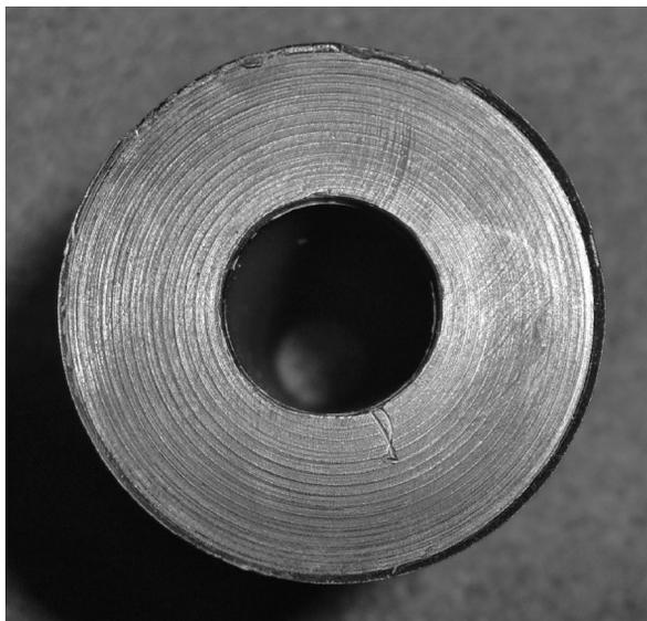
*Fig. 4 Wax grain after casting procedure*
