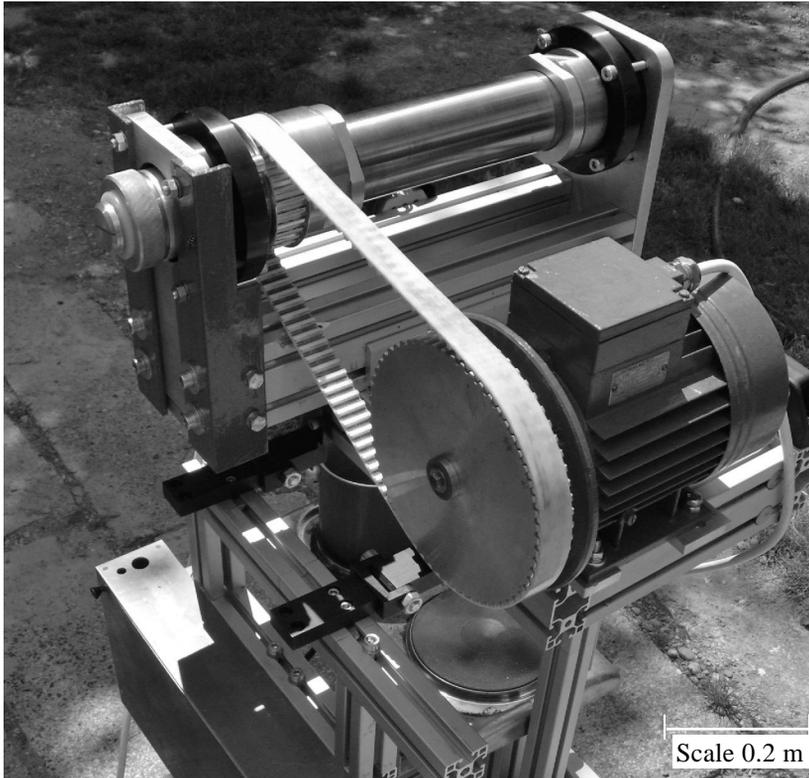
*Fig. 3 Rotary wax casting machine*
