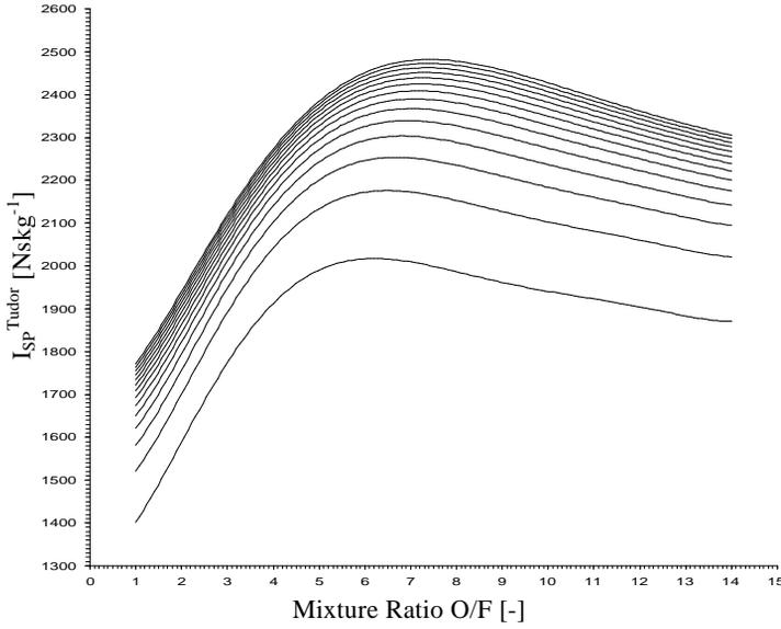
Fig.1 Theoretical values of specific impulse of HPH-12 mixture (nitrous oxide –  $N_2O/Wax$ ). These curves represent middle values of equilibrium and "frozen" flow
