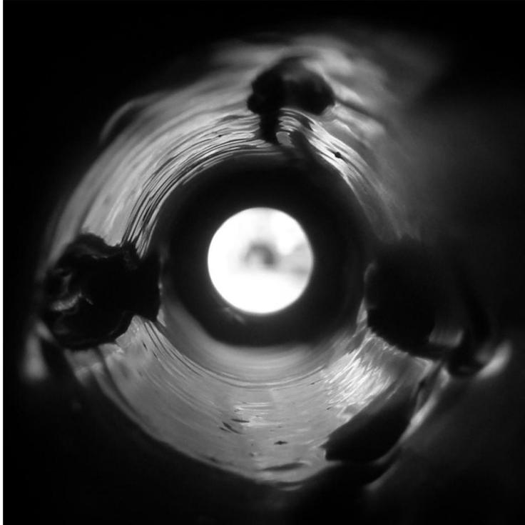
*Fig. 5 Wax fuel grain after first firing test. The hollows and depressions are caused by nitrous oxide injector malfunction*
