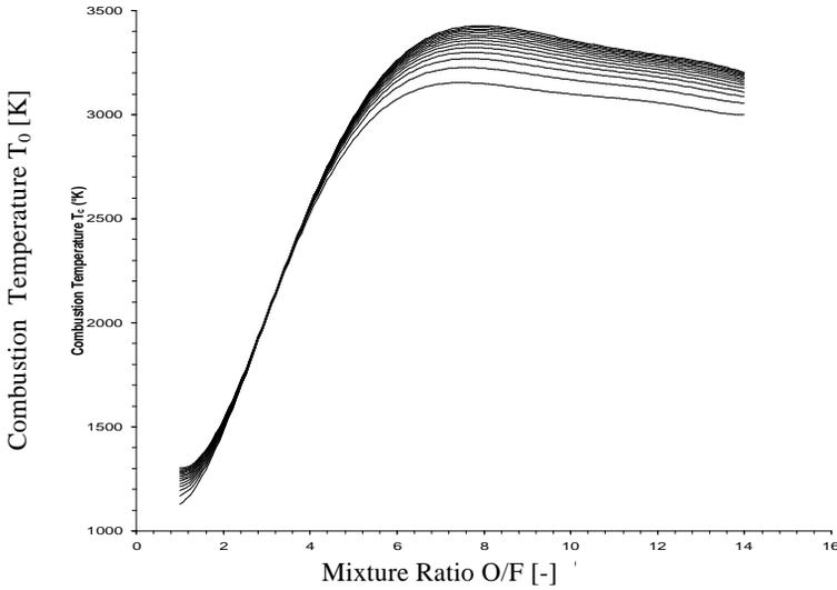
Fig.2 Combustion temperature of HPH-12 mixture
