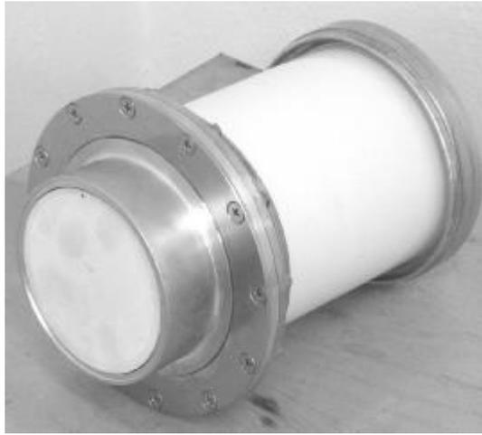
Fig. 6. View of fabricated axial vircator with adjustable distance between anode and cathode
