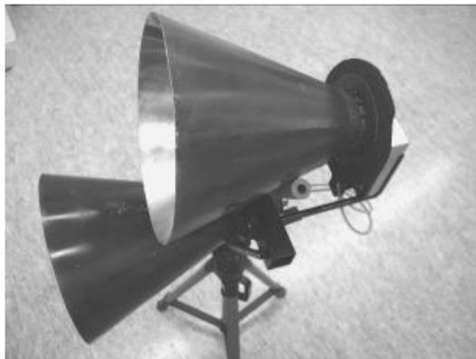
Fig. 13. Implementation of free space calorimetric measuring device
