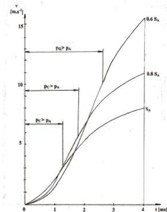
Fig. 2 Influence of  $S_A$  on the piston velocity  $v$
