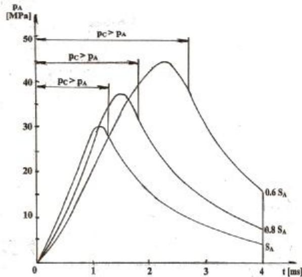
Fig. 3 Influence of  $S_A$  on the pressure in the gas cylinder  $p_A$
