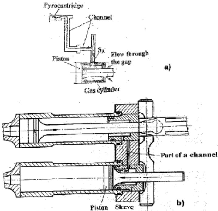
Fig. 1 Scheme of the pyro-recocking system
