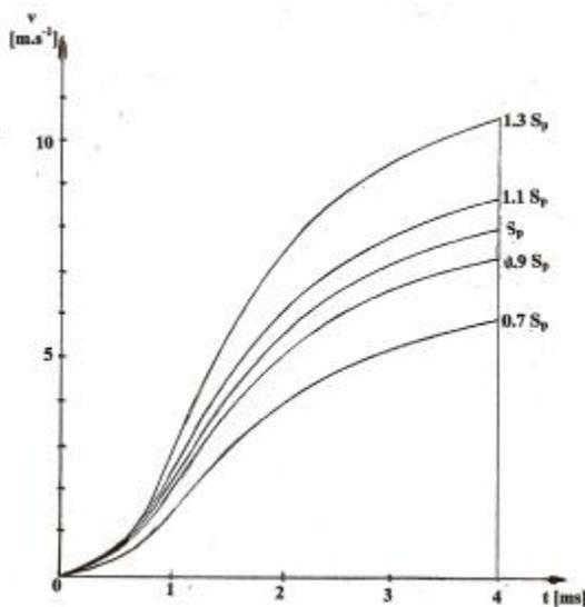
Fig. 4 Influence of  $S_p$  on the piston velocity  $v$
