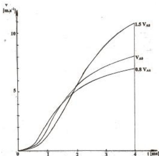
Fig. 5 Influence of  $V_{A0}$  on the piston velocity  $v$
