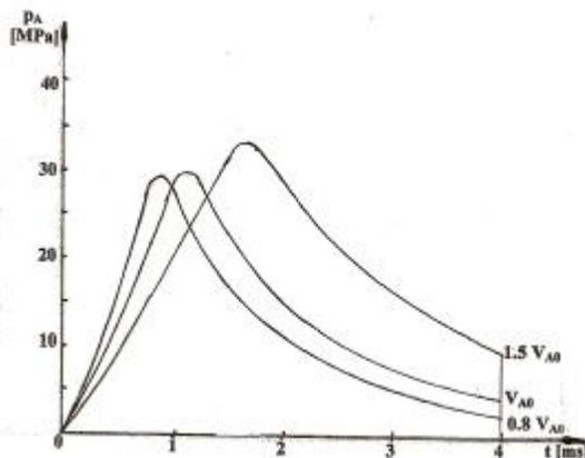
Fig. 6 Influence of  $V_{A0}$  on the pressure in the gas cylinder  $p_A$
