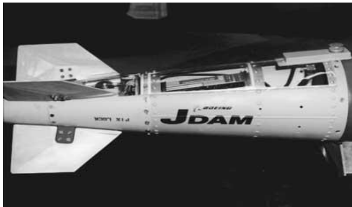
Fig. 13. The elements of the JDAM bomb guidance system associated with the Mk-83 bomb
