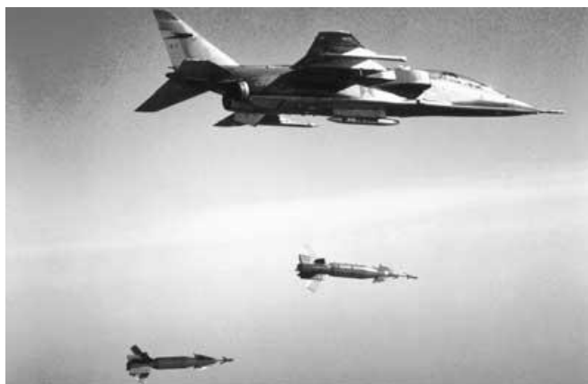
Fig. 9. Throw away the French bomb of BGL type from the Jaguar aircraft
