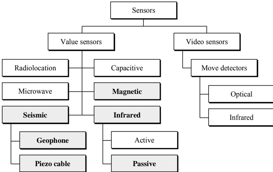
**Fig. 2** Basic UGMS sensors dividing for guarding of the area of interest
